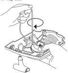
Stretch the line with the handle. Move your thumb and release the line. See the figure below.
